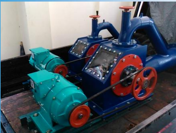
Pico with pelton turbine for higher head >50 m
